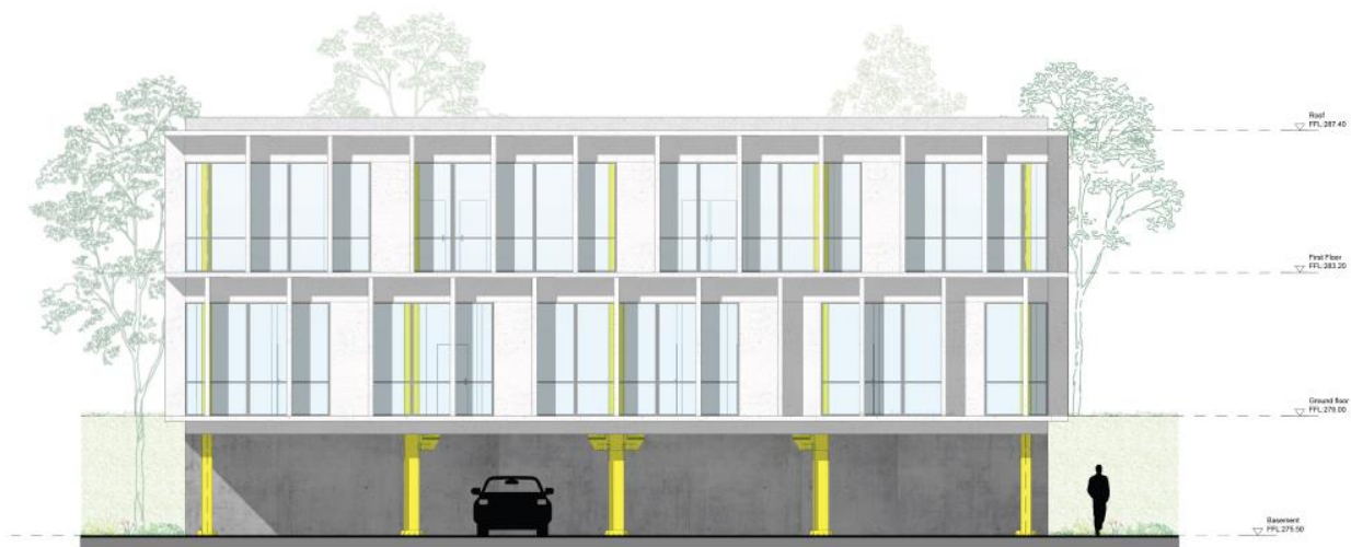
Figure 10: Second option for the façade system
