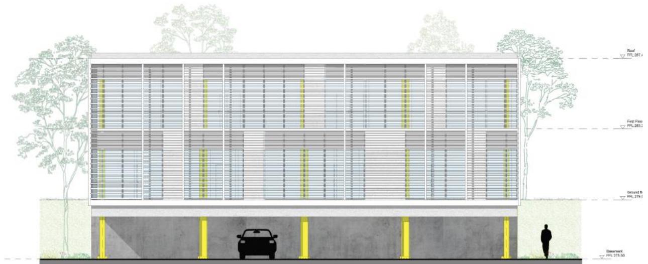
Figure 9: First option for the façade system (the adopted option)
